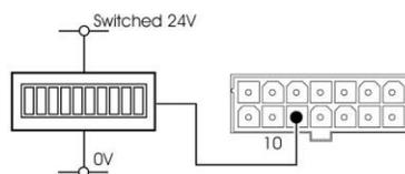
If you are using a bulb, the bulb can be connected directly between pin 10 and 0V (Highside) or pin 10 and switched 24V (Lowside). The bulb must be 12V with a maximum rating of 600mW when connected Highside and 24V with a maximum rating of 600mW when connected Lowside.
