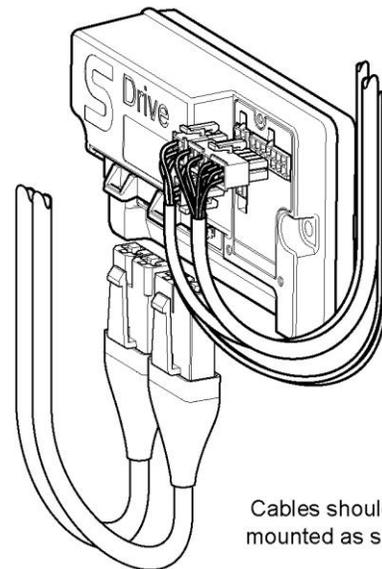
Cables should be mounted as shown
