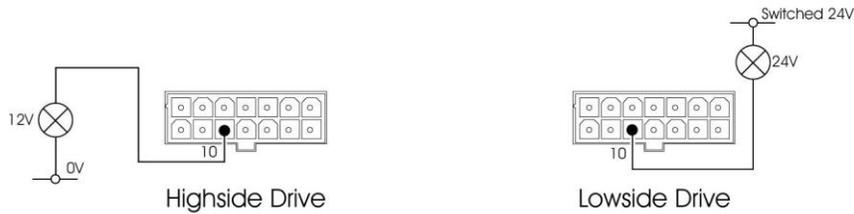
If you are using an Analogue 12V Status Indicator, it must be connected between pin 10 and 0V.
