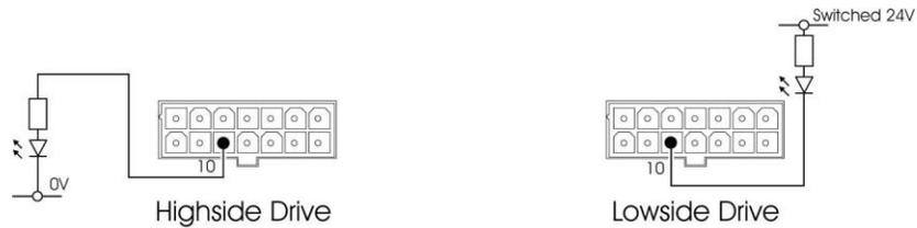
For each connection and indicator type the controller will require programming to suit. The parameter that will require adjustment is Status Output.
