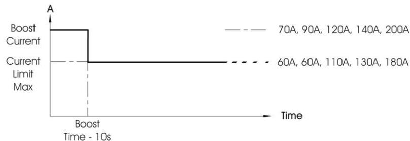
The drive boost current can be set in 1A steps between 10 and 140A but not less than the 'current limit max' setting, and the drive boost time to be altered in 1 second steps between 0 and 10 seconds.
